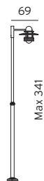
ART. 888 35W HIT, G12 Aluminium, 888AL Graphite, 888GR White, 888W EEI: A+
